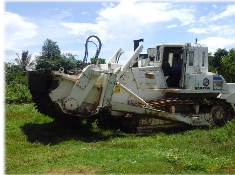
Demining Machine by KOMATSU Co.LTD
