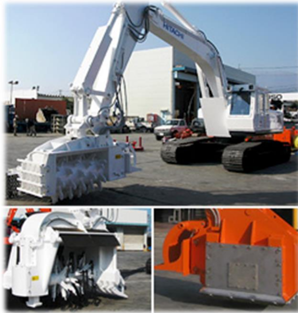
Demining Machine and attached cutter (by Nikken Co.LTD)
